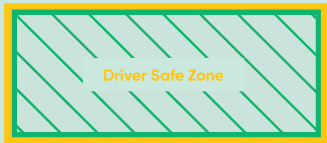
A designated area for drivers of truck and other vehicles to stand while their vehicle is being loaded. The driver will be segregated from vehicle and machinery operations with a barrier
